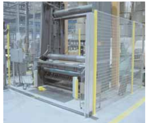
The paper slitter is powered down to a slow jog before the Flash-Fold opens for improved safety. The low profile Flash-Fold is mounted into the floor to allow unobstructed access to the paper slitter for easy loading and unloading.
