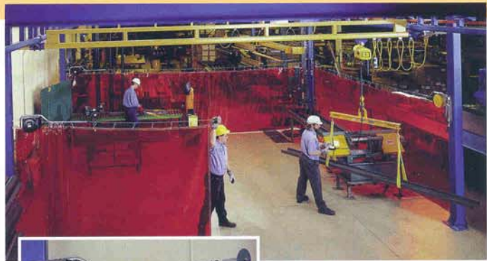
The X-Ten curtain stores on the cable guide, and the entire assembly can be rotated 180° for safe storage.
